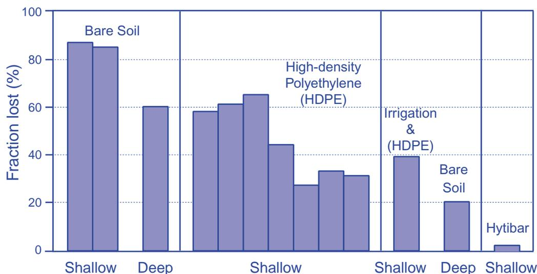
**Figure 1.** Comparison of total emission loss as affected by various fumigation practices. Shallow (25-30cm) and deep (50-70cm) indicate the injection depth.
